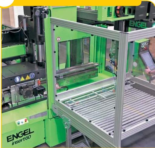
Our automated, state-of-the-art injection moulding production line forms the basis for manufacturing optical componentry. Most photometric optics are produced using either poly(methyl) methacrylate (PMMA) or polycarbonate (PC). These top-quality materials also demand flawless processing.
