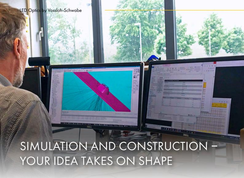
Based on your requirements, the first step is to simulate the lens geometry on the basis of the photometric targets. The simulation takes into account the LED data as well as the lighting requirements of the application.
