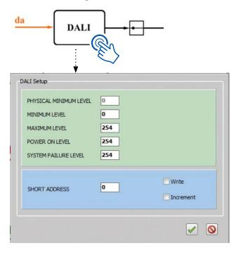
If available, the DALI parameters read-out with the "Read" command will be displayed here. The dimming range, start behaviour and error response can be adjusted. For every parameter, the DALI values 0 to 255 are available. The DALI device can also be given a DALI short address. By entering the short address and setting the check mark "Write" it becomes active. A click on ransfers the new parameters.
