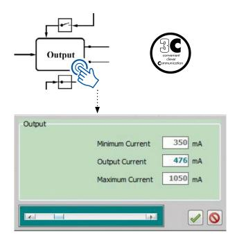
The physically possible minimum and maximum currents that were read-out with the "Read" command are displayed here. The desired operating current can be set within these limits. A click on will directly read-out the value to the DALI LED driver and close the pop-up window.
