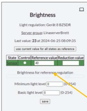
The reference values for light control must be set carefully and without unwanted light, otherwise the light control may not work.
