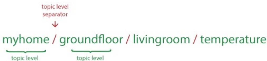
Customers can use different methods to interact with the VS Lina server MQTT interface and communicate with the VS Lina server.
