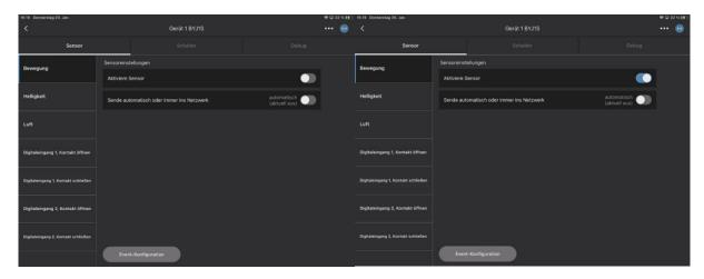
Figure 13: Step 1 (left) and step 2 (right) – activating the motion sensor
