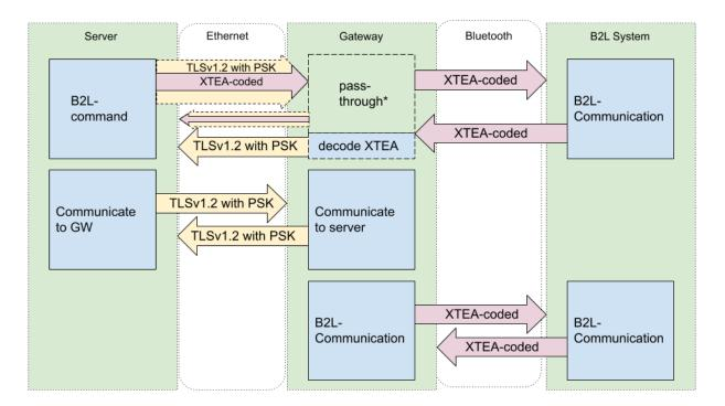
Figure 28: Visualization of the XTEA-algorithm in B2L
