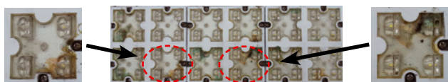
Figure 16: Example of an LED module (WU-M-425) operated in an environment with high concentrations of salt
