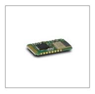
The signals necessary for proper operation of the module can be taken off at the soldering points provided for this purpose on the underside of the module. The corresponding contacts on the underside can be soldered.
